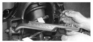
Replacing factory slotted alignment cams on the forward upper mount with cam lock plates. DO NOT OVER **TIGHTEN 40FT lbs max**
