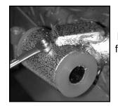
Install grease fitting in upper ball joint and control arms. Pump some grease in to
