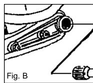
4) Loosen the height adjusting bolts until there is no longer any load on the torsion bars.
