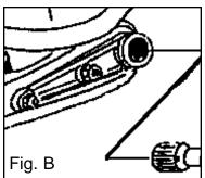
4) Remove the 2 bolts that hold the tension\compression rod and sway bar end link bolts.
