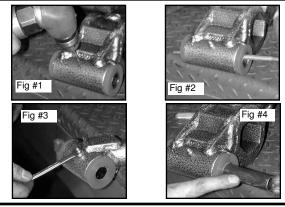
DJM recommends installing this control arm one side at of a time. Remove factory lower control arms. Keep factory bolts, nuts and sway bar hardware.
