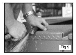
Trim about the same amount off the outer tie rod. The threads inside should be in good condition but check with the inner tie rod. If they don't spin on easily clean up the thread with a tap or a small grinding stone.
