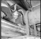
Remove the factory bump stop bracket from the frame drill 3/8" hole and and install bump stop to frame.
