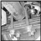
Place the new upper axle plates with the pin down on top of the axle. Install the 5/8" x 3-1/2" forward and the 5/8" x 4" to the rear, with one flat washers on top of the upper plate and one on the bottom of the axle locator.
