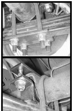
Remove stock rear bump stop. Find the 3/8 countersunk bolt. Apply loctite to threads and install the bump stop bracket with this hole facing forward. It will screw right in. Install urethane bump stop with the 3/8 bolt and nut provided. Do not forget to loctite the bolt.
