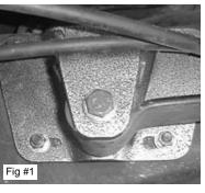
Apply some grease to the bushings and inside sleeves then attach new shackle on the frame mount and bolt in place with factory bolts (Fig #2). Shackle will install with bushings down and open side forward. The hole farthest away from bushing will lower truck more than the closer hole. Now raise the rear axle high enough to align the spring eye and shackle. Insert the remaining bolt and install nuts.
