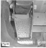
Install rear wheels and torque lug nuts. Remove jack stand and floor jack. Check the height of the rear. You can change the height by moving the spring to the other hole in shackle. When satisfied with the height, install new shocks. Tighten all bolts.
