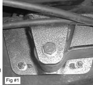
Apply some grease to the bushings and inside sleeves then attach new shackle on the frame mount and bolt in place with factory bolts (Fig #2). Shackle will install with bushings down and open side forward. The hole farthest away from bushing will lower truck more than the closer hole. Now raise the rear axle high enough to align the spring eye and shackle. Insert the remaining bolt and install nuts.
