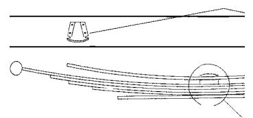
Working on one side at a time, remove the u-bolts holding the springs to the axle. To keep spring pack together while removing over load, use two large C-clamps, placed close to center bolt on leaf spring and tighten.
