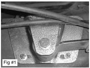
the hanger before bolting the hanger to the frame.) See fig #1 for typical hanger installation.
