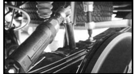
Now remove the stock shackle. The upper bolt will hit the frame as you pull it out, so with the u-bolts off, you can move the spring out enough to get the bolt out. The new shackle will replace the factory shackle using factory hardware. Apply some grease to the busings. Wait to tighten shackles until installation is complete.
