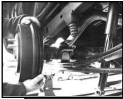
Install new U-bolts and spring plates (5 hole) on the bottom of the springs. Tighten the nuts on the u-bolts to hold axle in place.
