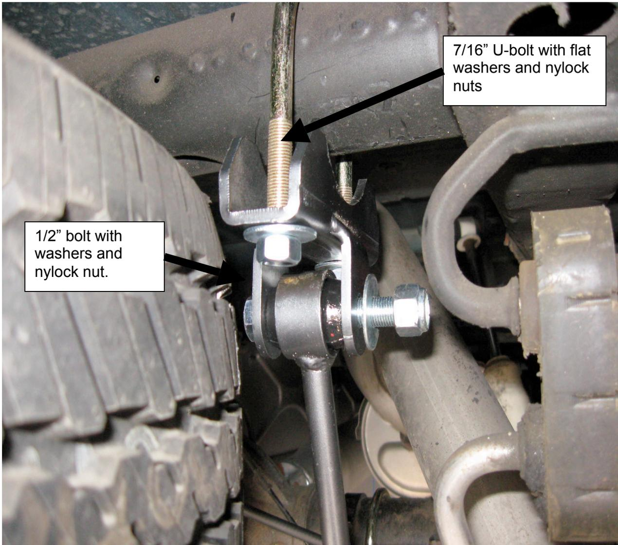
2. Loosely assemble the upper saddles on the cross member in front of the spare tire as shown. Make sure to move any electrical wires that may interfere with the mounting location (both sides of the spare) on the cross member. Attach end link as shown with the head of the bolts towards the center of the truck. Do not tighten at this time.
