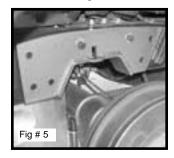
Install remaining 7/16" bolts and tighten.
