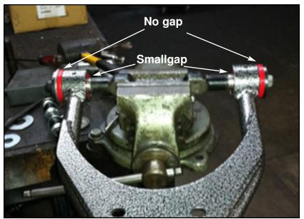
Now that the control arm is mounted you need to check for end play. Your kit will come with 2 washers that will help you with the end play. After tightening the bolts there should be no gap between the large thick washer and the bushing but still maintained the cap on the sleeve and shoulder of the mounting shaft. If this is how you control arm mount look just remover the bolts and loctite and you ready to reinstall them on the truck
