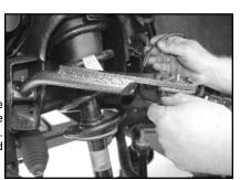
Check all bolts are tight and grease all fittings. Test drive. Align to factory specs.
