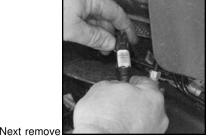
the ball joint from the spindle. taping the side of the spindle with a mallet will usually loosen the taper. A pickle fork could be used but may damage
