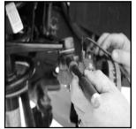
Unbolt the arm from the frame. Note where the the factory cams are adjusted. You will install them with the new arm in the same position. The bolts are installed from the inside out. There is little clearance to remove the bolts. Wiggle them around the spring to remove.
