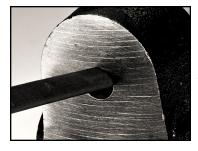
On 2016 and 17 steel spindle only. there is a bur on the upper ball joint tapper. You can remove this with a file or rotory tool. Pre fit the ball joint before installation
