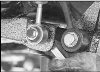
10) Re-install the strut, sway bar with the new bolts supplied.
