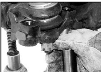
4) The ball joint on Toyotas can be removed by removing the mount from the spindle. This makes it much safer to press the ball joint out of the mount on a H-frame press. Remember the ball joint is going to be re-used so it's important not to damage the boot.
