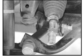
12) Remove the tie rod end completely. We want to cut 1/4" off the end. A cut off wheel does a really good job and won't damage the threads. The purpose is to ensure enough toe adjustment. This will not cause a problem if the truck has to be returned to stock.
