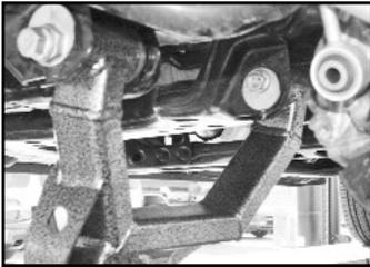
9) Hang the arm on the truck. Hand tighten only after the arm is completely installed, line up your marks then tighten.
