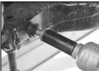
2) Remove the strut bolt. The bolt is not re-used on the new control arm but keep it with the original one if you chose to put it back to stock sometime in the future.
