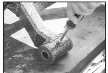
7) Zerk fitting need to be installed in the new arm. The fittings are left out because they could easily get broken off in shipping. The holes are drilled and tapped, so install them just before installing the arm.
