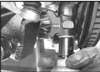
11) We installed the balljoint to the mount before bolting the mount to the spindle. Before bolting the mount to the spindle use some thread lock at this point.
