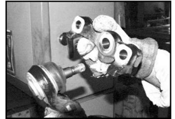
5) The balljoint is now freed from the mount with no damage to the threads or boot. We use a scrap piece of tubing that fits the ball joint well to press it out of the control arm. A little extra time on your setup will insure you do not damage anything.
