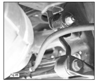
extender with the factory shock mount. Using the  $1/2^{\circ} \times 1^{\circ}$  bolts attach shock extender to factory shock mount, use a flat washer and lockwasher on each bolt. Nuts will go on the inside. Use one  $1/2^{\circ} \times 1-1/4$  bolt through the cross brace and attach to the threaded reinforcement plate on the back side of the factory mount. Attach shock to new shock extender using original bolts.
