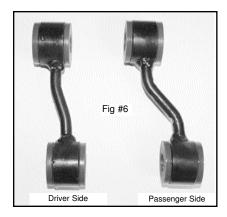
Apply some grease to the bushings and bolt the driver side end link to the factory upper mount using factory hardware. The lower end is offset to the passenger side. Bolt the sway bar to the outside of the endlink using 1/2" x 2-3/4" bolts (Fig # 7).
