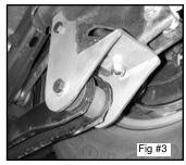
Remove factory orange bump stop and cut off first ring. Reinstall bump stop.
