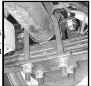
Place the new upper axle plates with the pin down on top of the axle. Install the 5/8" x 3-1/2" forward and the 5/8" x 4" to the rear, with one flat washers on top of the upper plate and one on the bottom of the axle locator.
