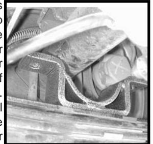
Install new U-bolts and spring plates (5 hole) on the bottom of the springs. Cross-torque u-bolts. Over tightening may bend spring plates.
