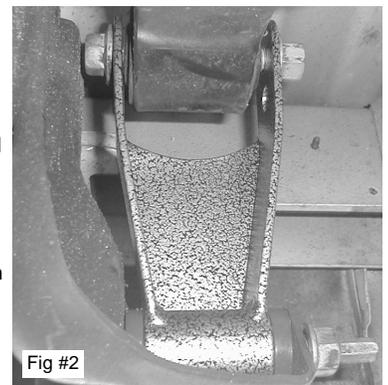
Install rear wheels and torque lug nuts. Remove jack stand and floor jack. Check the height of the rear. You can change the height by moving the spring to the other hole in shackle. When satisfied with the height, install new shocks. Tighten all bolts.
