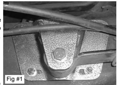
Apply some grease to the bushings and inside sleeves then attach new shackle on the frame mount and bolt in place with factory bolts (Fig #2). Shackle will install with bushings down and open side forward. The hole farthest away from bushing will lower truck more than the closer hole. Now raise the rear axle high enough to align the spring eye and shackle. Insert the remaining bolt and install nuts.
