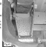
Remove stock bump stop and replace with new shorter stop.
