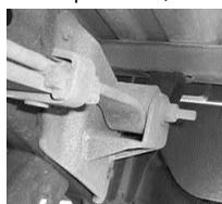
Apply some grease to the bushings and inside sleeves then attach new shackle on the frame mount and bolt in place with factory bolts (Fig #1). Shackle will install with bushings down and open side forward. The hole farthest away from bushing will lower truck more than the closer hole. Now raise the rear axle high enough to align the spring eye and shackle. Insert the remaining bolt and install nuts.
