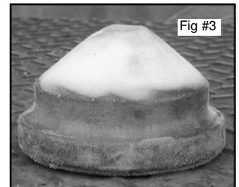
Remove factory orange bump stop and cut off first ring. To give the bump stop a more custom look we modified it on our belt sander. Reinstall bump stop.
