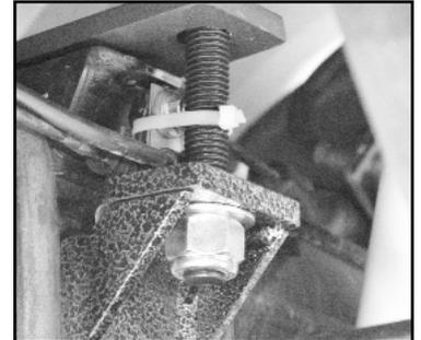
Place the new upper axle plates on top of the axle, align pin with hole on axle. Install the 5/8" bolts provided (4" front 4.5" rear some axles will use 4.5" on both) with one flat washers on top of the upper plate and one on the bottom of the axle locator. Check pinion angle.
