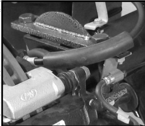
Tighten U-Bolts and axle bracket bolts.
