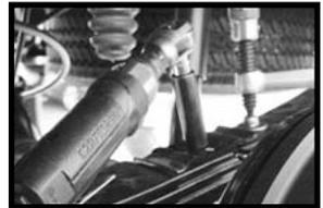
On the driver side, unbolt the factory shackle. Leave the front bolt in place so you won't have to move the gas tank. Reverse center bolt the same as on the passenger side.
