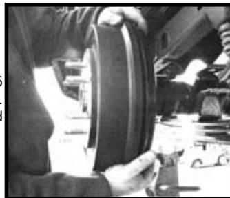
Place the new upper axle plates on top of the axle, align pin with hole on axle. Install the 5/8" bolts provided with one flat Washes on top of the upper plate and one on the bottom of the axle locator. Raise the axle to ride height and adjust pinion angle as needed.
