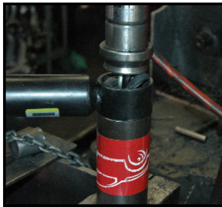
Press the bushing out. It comes out easy
