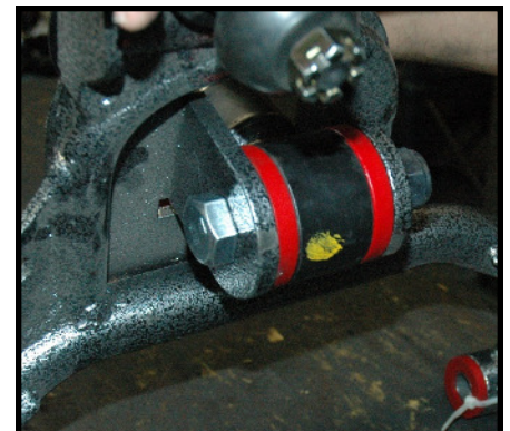
Bolt on the control arm with M20 X 100mm bolt and nut
