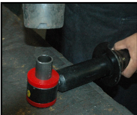
Tap the outer sleeve with a mallet
