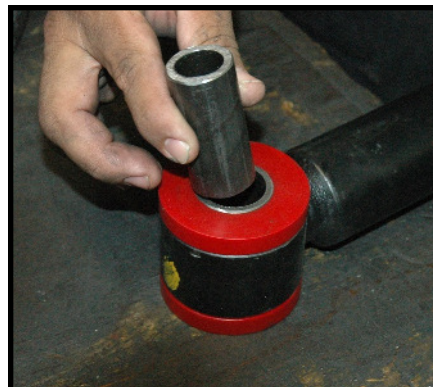
The inner sleeves just slides in
