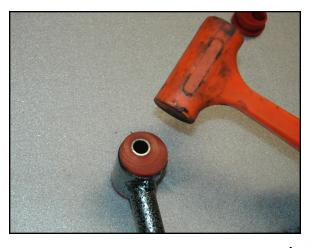
Make sure your holes are lined up and gently tap in the sleeves. Let it dry over night. Install with the supplied cam locks in you control arms kit and do not over tighten follow the instructions that came with the control arms.
