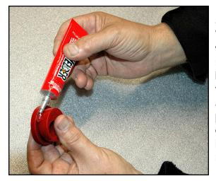
Second a small amount of Welder goes and long way so you don't need much. Put a thin coat on both the bushing and control arms. Let is set up about 10 minutes and press the bushing in. You can do this by hand or a little pressure with the mallet.
