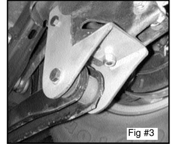
Remove factory orange bump stop and cut off first ring. Reinstall bump stop.
