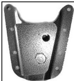
Remove the rivets holding spring hanger to the frame. This can be done with a air chisel or drill out rivets. With new bolts supplied, attach spring to hanger and install nuts. Do not tighten nuts. Mount your new DJM Spring hanger in original holes on the frame with hardware provided, torque bolts to 55-60 ft/lb. Gas tank will need to be moved to gain access to bolts on driver side. There are two holes in the hanger to bolt the springs, this will give you some adjustment.
