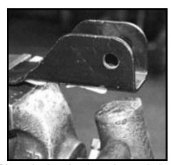
Place the bracket in a vice and give it a couple of good hits. We want to create and angle that will help us with alignment
