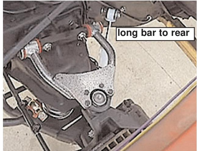
Work on one side at a time. Loosen the nuts holding the mounting shaft to the frame. Remove the alignment shims from behind the mounting shaft. Keep the shims together and note forward and rearward. When you install the new arms, place the shims the same way there were removed.
