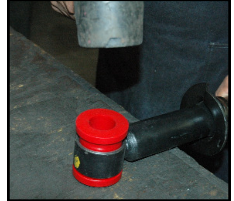
Tap the new bushing in with a mallet
