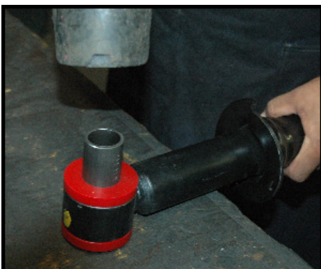
Tap the outer sleeve with a mallet
