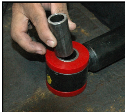
The inner sleeves just slides in
