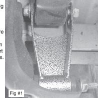
Remove stock bump stop and replace with new shorter stop.
