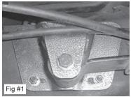
find it easier to attach the spring to the hanger before bolting the hanger to the frame.) See fig #1 for typical hanger installation.
