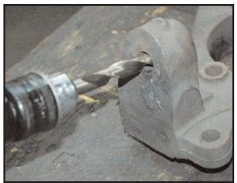
A good way to accomplish the material removal is to pass a 1/2" drill though the hole. Make sure not to wabble the drill that will effect the taper. You just want to open the very bottom of the small side of the taper. You also can use a rat tail file. Remember not to contact the taper just the very bottom on the hole
