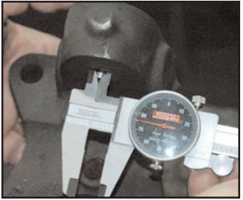
The spindle on your Chevy truck is about .020 smaller than the stud on the ball joint. You can use a die grinder, drill or rat tail file to open the hole
