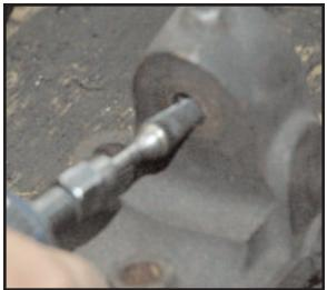
There are many ways to open up the hole that the stud passes though. The photo shows using a die grinder. When using a die grinder you want to make sure not to change or contact the taper in any way. Remove a small amount of material keeping the grinder straight on the small side of the hole until the ball joint drops in.
