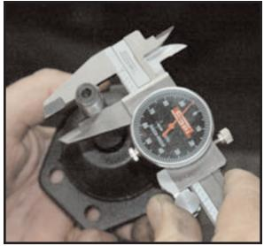
When installing 6136 ball joint a small modification needs to be done. There is a .020 difference between the stud of the ball joint (threaded part) and the spindle. This is a very small difference and can be done in a few minutes.
