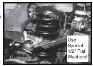
with new custom  $\ensuremath{\ensuremath{\%^{\text{"}}}}$  flat washers placed between bolt and bushing and tighten.
