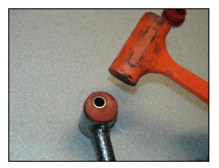
Make sure your holes are lined up and gently tap in the sleeves. Let it dry over night. Install with the supplied cam locks in you control arms kit and do not over tighten follow the instructions that came with the control arms.
