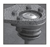
Unbolt brake line and remove factory upper arm. Apply grease to the sides of the bushings and install using factory hardware. Align ball joint with spindle, use 2 flat washers as spacer between spindle and nut. Tighten and install new cotter pin.
