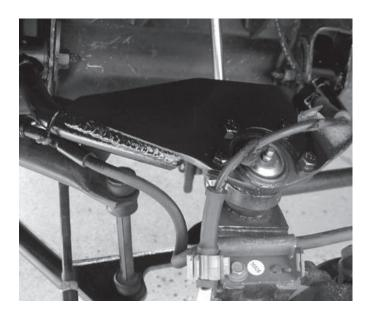
There are 2 small holes in the plate behind the ball joint. They are for the factory plastic rivet used to hole the ABS sensor.
