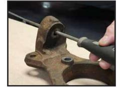
On 2016-2018 steel knuckle only. There is a small burr on the upper ball joint tapper. This can be removed with a file or a die grinder. Test fit the upper ball joint to make sure there is no interferance.
