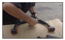
Install the upper ball joints and grease fitting, Lower ball joints are installed at the factory and only the grease fitting need to be installed
