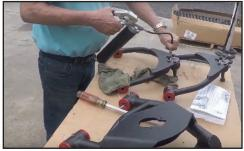
Lube the fittings make sure the predrilled grease holes, grease fitting and twin sleeve accept the grease and moves smoothly
