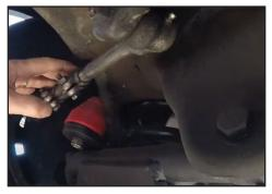
Make sure to point to tie rod sleeve so the bolt heads are away from the bump stops make sure there is no contact
