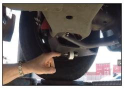
After the coil spring is compressed and in position install the shock and you will be able to remove the jack
