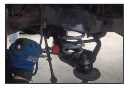
Install the control arms and coil, Caution needs to be taken when compressing coil springs make sure everyone is out of the way and safe.
