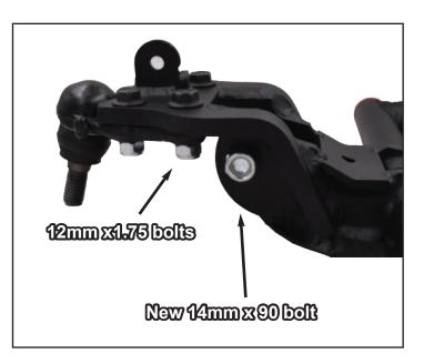
Check all hardware has been tightened. When installation is complete, test drive vehicle. A front end alignment is required. Align to factory specifications.
