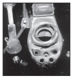
Remove the two nuts on the outer end of the lower arm that hold the spindle mounting bracket and remove bracket. The two studs are pressed into the bracket. When all these parts are removed the lower arm will look like the picture.
