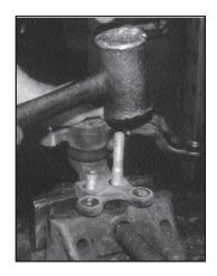
Remove the studs in the spindle-mounting bracket. This can be done on a press or tap them out using a mallet and bench vice.
