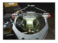
Now that the control arm is mounted you need to check for end play. Your kit will come with 2 washers that will help you with the end play. After tightening the bolts there should be no gap between the large thick washer and the bushing but still
