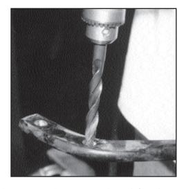
Use the same procedure to remove the studs from the T\C rod. Use a 9\16" bit and drill out the holes for the new bolts.
