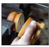
Next install new rear coil springs using factory isolators. Raise the axle until both coils are fully seated. Tension must be maintained on the coils until the installation is complete. You can support the axle with jack stands or install wheels and set vehicle on the ground.
