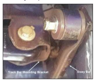
The d-bushing on the driver side must be moved over on the frame about 1" (Fig #4). Ubolt driver side bracket, slide the bracket to the passenger side. Mark and drill two 3/8" holes and bolt on with 3/8" x 1" bolts
