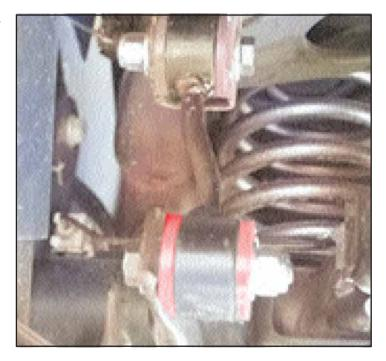
Apply some grease to the bushings and bolt the passenger side end link to the factory upper mount using factory hardware. The lower end is offset to the passenger side. Bolt the sway bar to the outside of the endlink using 1/2" x 2-3/4" bolts (Fig # 8)
