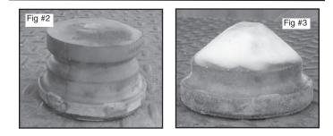
Remove factory orange bump stop and cut off first ring. To give the bump stop a more custom look we modified it on our belt sander. Reinstall bump stop.
