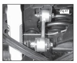
Apply some grease to the bushing and bolt the driver side end link to the factory upper mount using factory hardware. The lower end is offset to the passenger side. Bolt the sway bar to the outside of the end link using  $1/2^{\circ}$  x 2-3/4° bolts (Fig # 7).
