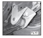
Unbolt trailing arms from under the axle. Bolt the new DJM Trailing arm bracket to the axle mount using the original holes. Attach with  $1/2^{\circ} \times 1-1/4^{\circ}$  bolts. Bolt trailing arm to the new bracket with  $9/16^{\circ} \times 4-1/2^{\circ}$  bolts. Tighten bolts for brackets then trailing arms. Do not over tighten trailing arm bolts. (Fig # 2& 3).
