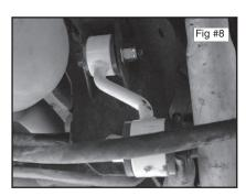
Apply some grease to the bushing and bolt the passenger side end link to the factory upper mount using factory hardware. The lower end is offset to the passenger side. Bolt the sway bar to the outside of the end link using  $1/2^{\circ} \times 2-3/4^{\circ}$  bolts (Fig # 8)
