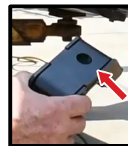
Center hole goes to front of truck.
